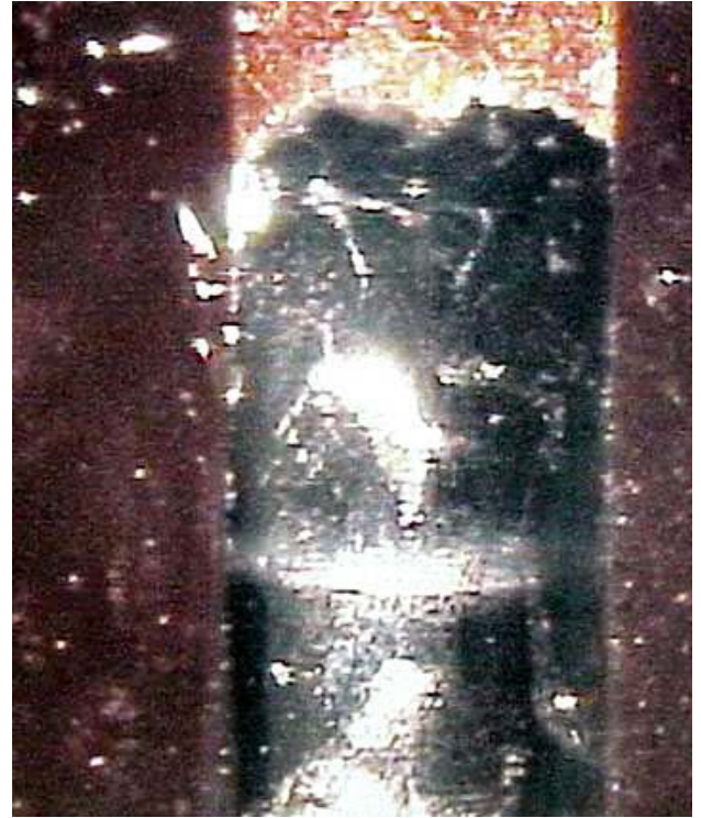
( Figure 9, using the dross elimination material, note improved wetting)
